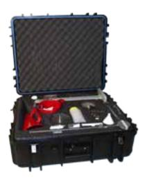
The Model IND SlurryTest Kit is a field transportable kit containing testing equipment designed for measuring the physical and chemical properties of slurries formulated in the field. This kit allows laboratory-quality measurements of funnel viscosity, plastic viscosity and yield point, specific gravity/density, pH, water hardness, sand content, and water loss (filtration) properties.
