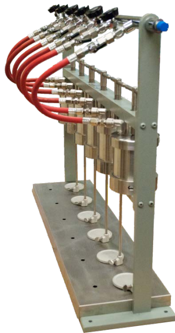
Figure 10-9 Six Unit Filter Press w/Manifold
