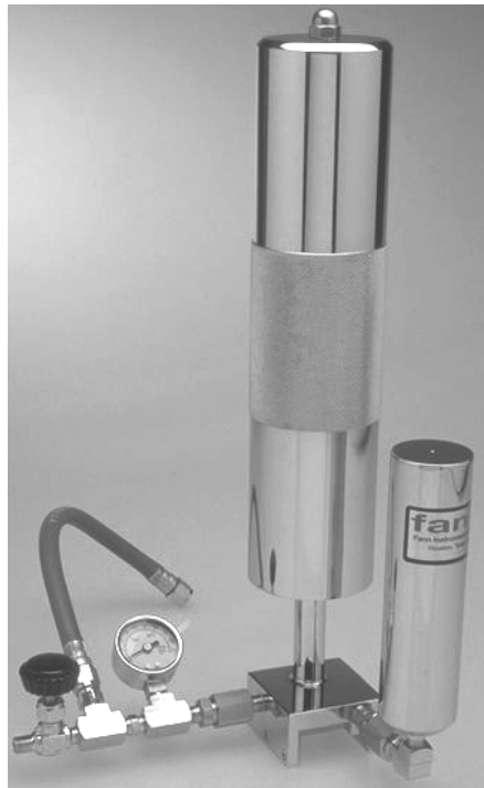
Figure 10-6 Dead-Weight Hydraulic Assembly
