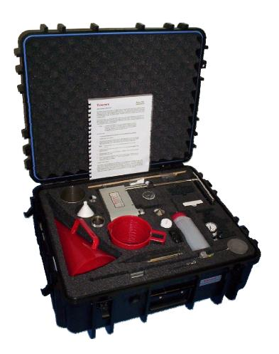
Drilling Fluids are used in many industrial applications: water well horizontal drilling, directional drilling (HDD), drilled shaft applications, and mining applications. It is essential to control various properties of drilling fluids (also called "slurries") during the process. This is accomplished by measuring the physical and chemical properties of the drilling fluids.
