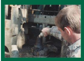
**Application of Inpol-Lube** for a (3 inch to 6 inch diameter down-hole hammer).
