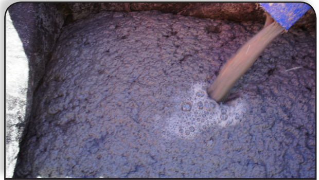
2 Flocculant applied to cone underflow
