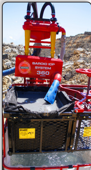
3 Water separates from flocculated solids
